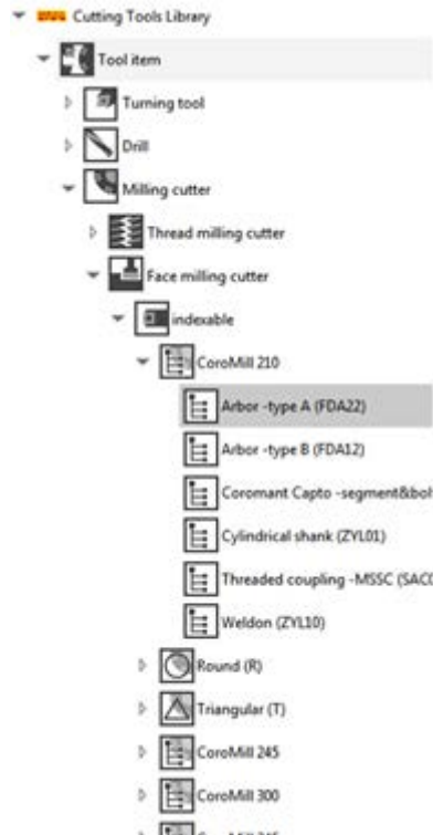
Example of branches in the GTC structure.
